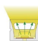
T2014 Top View 20x14mm PCB Width - 10mm
