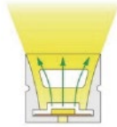
T1212 Top View 12x12mm PCB Width - 8mm
